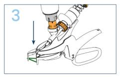
Place the ring over the tail or scrotum and release the trigger. The stretched ring will hold the device in position while you depress the injector.
