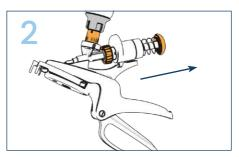
Tilt the applicator down and back to release the ring in position.
