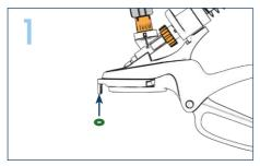
Press ring onto the three front pins on the Numnuts device.
