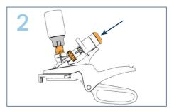
Fully depress and release the injector button two or three times until fluid is present in fluid junction.
