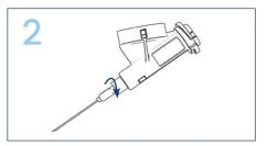
Remove the needle using needle nose pliers, if necessary. Screw needle on to the fluid junction until finger tight.
