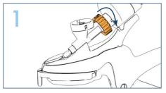
Detach the fluid junction and needle from the injector by rotating the orange lock nut and sliding the fluid junction forward.
