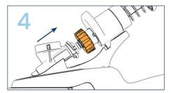
Slide the fluid junction back into the injection mechanism and secure by turning the orange lock nut until finger tight.
