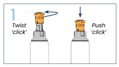
Place the bottle on a flat surface. Whilst holding the grey collar of the Quick Change Cartridge, twist the orange cap to break the seal. You will hear a 'click'. Now push the orange cap down squarely to broach the bottle. You will hear a 'click'.
