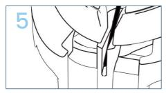
Check the position of the needle. When injector is fully retracted, the needle tip should be about 2 mm hidden inside the front pin.
