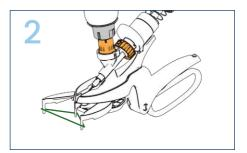
Squeeze the trigger to fully open the ring.
