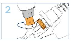
Place the Quick Change Cartridge onto the fluid junction. Twist the orange collar until tight. Over-tightening can crack the fluid junction.
