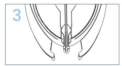
Squeeze the device trigger to open the front pins. Place the needle into the front pin slot and fluid junction lugs into the slots in the device.
