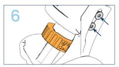
To adjust needle position, loosen the two screws under the injector using a 2.5 mm hex key. Move accordingly and tighten to secure.
